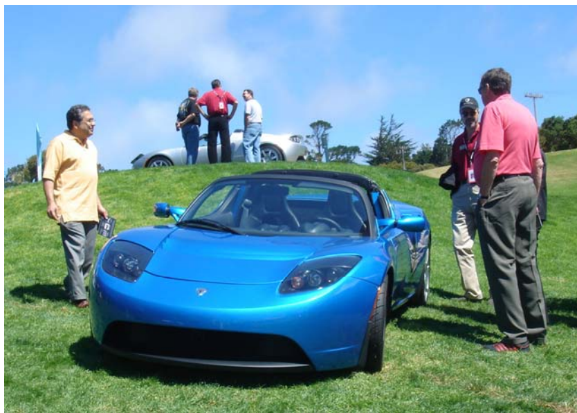
Fig. 3: The "Tesla Roadster" BEV: Vehicle efficiency 2.18 km/MJ and 300 km per charge (can be fully recharged "overnight" according to the manufacturer) [ http://www.teslamotors.com ]. 0-100 km/h in 5 seconds. Estimated well-to-wheel efficiency based on natural gas as primary energy source is 1.14 km/MJ (assuming a well-to-tank efficiency of 52%). Based on a Li-Ion battery pack. The purchase price is approximately $110,000 and the delivery time is currently up to 15 months.
